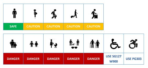
If regular use by user types with the risk classification of caution or danger is anticipated, than we recommend that the optional detection sensors are fitted, all parameters are set to the optimum level of protection and additional safety signage may be required.
