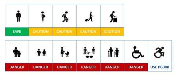
If regular use by user types with the risk classification of caution or danger is anticipated, than we recommend that the optional detection sensors are fitted, all parameters are set to the optimum level of protection and additional safety signage may be required.
